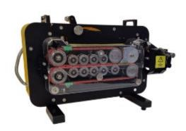
The Hurricane has been designed to maximise protection for micro cables with a compliant double drive concept, backed by the latest technology in servo controls to provide precise control of torque and speed. Single person operation with safe, easy to operate ergonomic controls combines with low maintenance and high reliability to form the machine's key features. The Hurricane is adjustable to suit a wide range of cable diameters from 2.5mm to 16mm.
